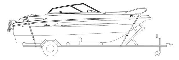
Image: Attaching the boat to the trailer.
