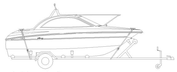
Fastening the boat onto the trailer
