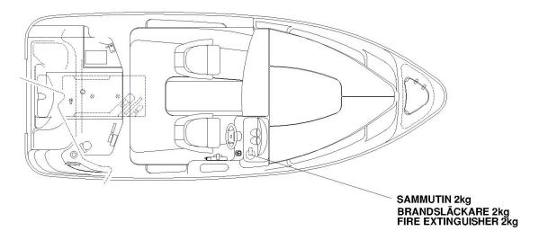
YAMARIN 56 Hard Top. Location and rating of portable fire extinguisher
