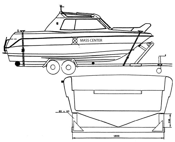
Fastening the boat onto the trailer
