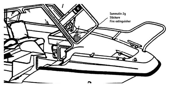
YAMARIN 59 Cabin. Location and rating of portable fire extinguisher
