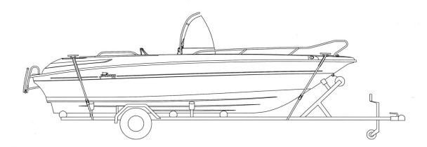
Tie the boat properly before starting the transport. Fastening belts located at the bow should be directed "down-back" and fastening belts located at rear should be directed "down-front". Do not leave any loose equipment or extra load to boat when it's transported. Take seat cushion away and close the hatches properly.
