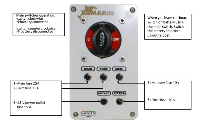
Fuses number one, two three, four and five are automatic. In case of short-circuit current automatic fuse will trigger itself. You can "prime" it again by pressing it back in. If the automatic fuse releases itself again you have a short-circuit in your electric system or in some component, in which case please do contact an authorised service shop.
