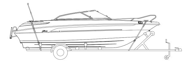
Tie the boat properly before starting the transport. Fastening belts located at the bow should be directed "down-back" and fastening belts located at rear should be directed "down-front". Do not leave any loose equipment or extra load to boat when it's transported. Take seat cushion away and close the hatches properly.
