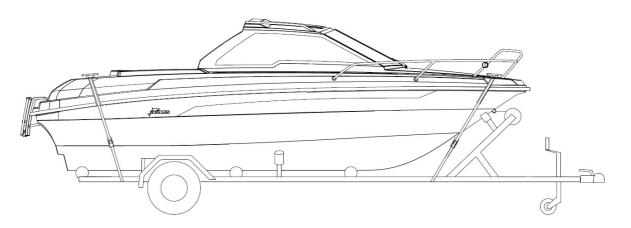
Image: Attaching the boat to the trailer.
