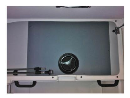
Image: The fresh water tank filling hole underneath the maintenance hatch.
