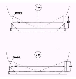
Only use reputable lifting companies or boat yards with sufficient lifting capacity. In addition to the boat's own weight (please refer to technical specification), also take into consideration the accessories and other possible loads on the boat.
