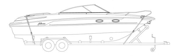
Tie the boat properly before starting the transport. Fastening belts located at the bow should be directed "down-back" and fastening belts located at rear should be directed "down-front". Do not leave any loose equipment or extra load to boat when it's transported. Take seat cushion away and close the hatches properly.
