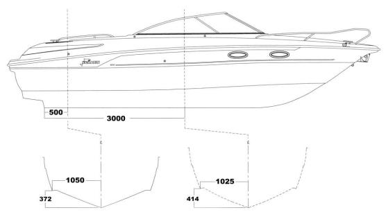
Only use reputable lifting companies or boat yards with sufficient lifting capacity. In addition to the boat's own weight (please refer to technical specification), also take into consideration the accessories and other possible loads on the boat.
